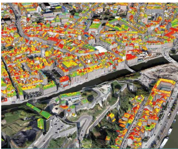
AERIAL THERMOGRAPHY - SOUTH OF LA CORBEILLE AND RUE NOTRE DAME
